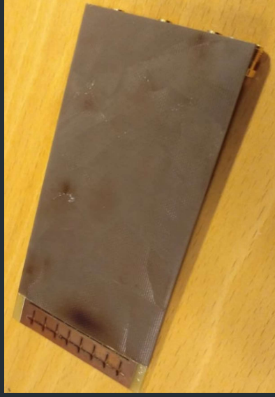
“Substrate-Insensitive Phased Array with Improved Circularly-Polarized Scan Angle for 5G Mobile Terminals”
